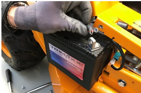
Disconnect the negative terminal of the battery. Remove ignition key.
