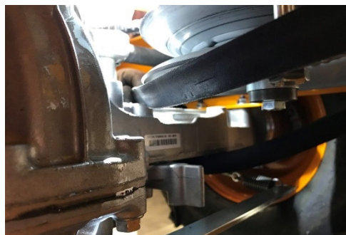
Twist blade belt in order to come through the rear axle and engine belt pulley.
