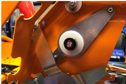
Blade switch-on lever, installation: Step #4 (continued)
