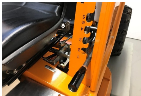
Place the mower deck height adjustment element on the lowest position "1".
