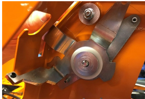
Blade switch-on lever, installation: Step #4 (continued)
