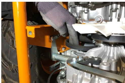
Pull the blade belt to the rear, slightly off the engine belt pulley.
