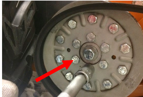
Detach belt pulley → inner screws
