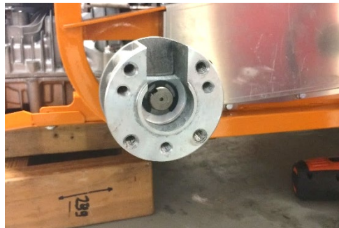
Prop up vehicle right rear and take off rear wheel
