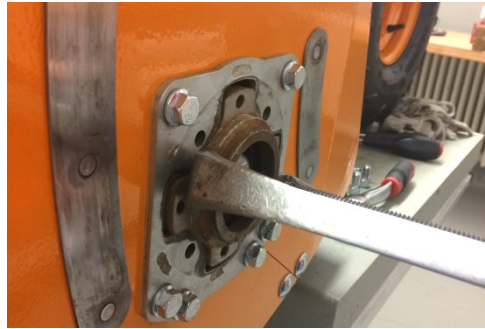
Twist and pull off bearing block → knock-out bearing
