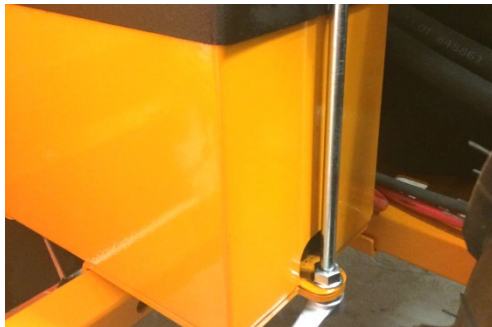
Remove battery → first disconnect the negative terminal
