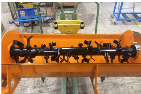
Flail shaft installed
