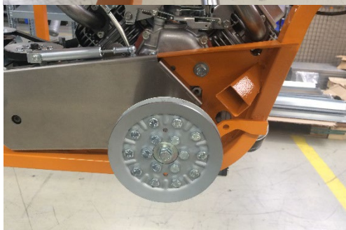
Belt tensioner for reduction gearing View from the outside
