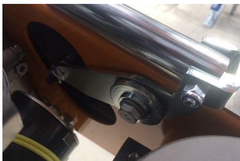
Belt tensioner for reduction gearing – view into the frame
