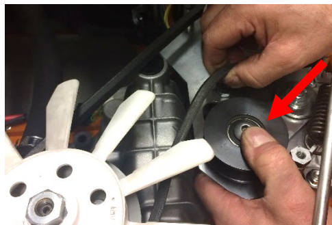
De-tension the belt tensioner by hand and take off the belt
