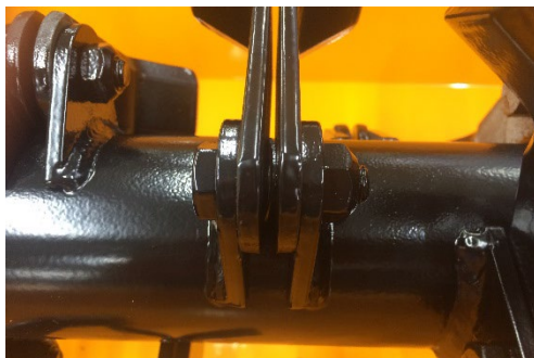
Screw must completely fill out the nut
