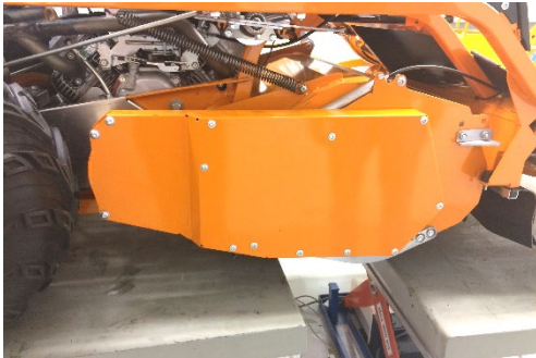
Detach cover → pay attention to the spacer sleeves
