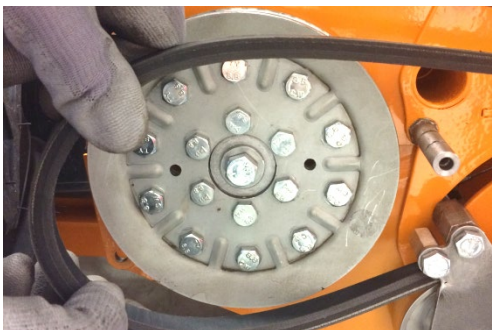
Take off V-belt of the mower unit drive
