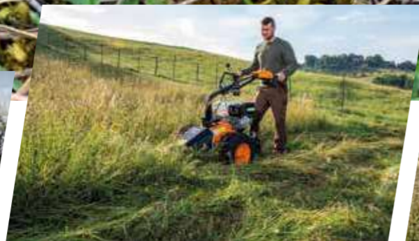
Gentle cut with double knife cutter bar
