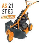
AS 2-stroke engine, 165 ccm, EasyStart. Rated power 4.0 kW (5.4 hp), max. 4.4 kW (6.0 hp). Cutting height 55 - 80 mm, cutting width 51 cm.
