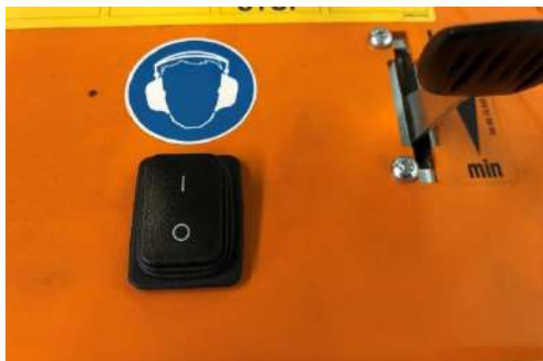
AS 901 with new start switch.
