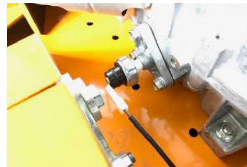
AS 701 engine (oil pressure switch)
