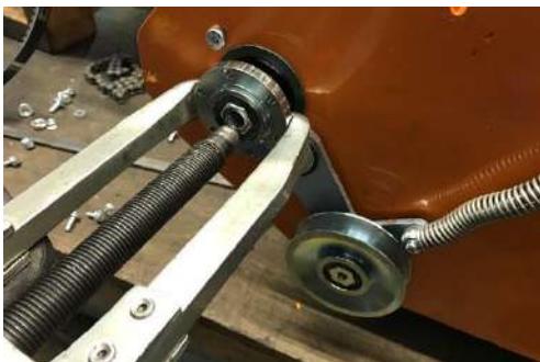
Pull the belt pulley off of the belt pulley hub.
