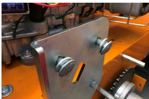
Insert carriage bolts with washers.
