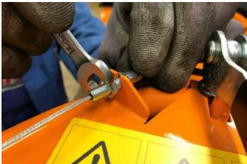
Mount the cable stop.
