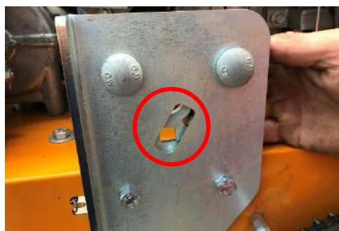
Square hole of the sprocket is centred in the aperture.
