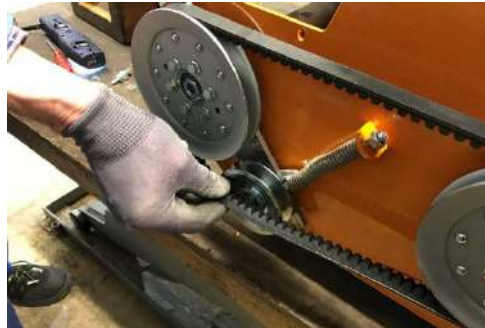
Take belt off of the tension pulley.
