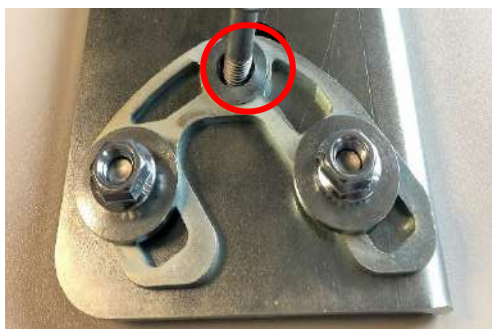
Do not forget the disc
