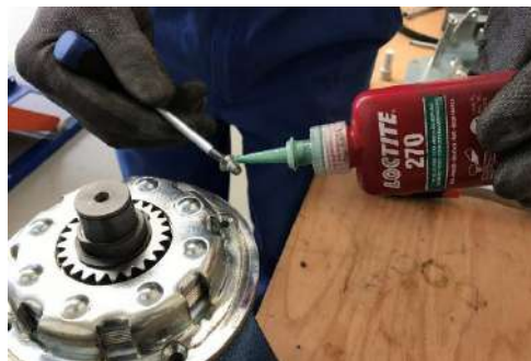
Secure the screws of the clutch basket with Loctite 270. ⚠
