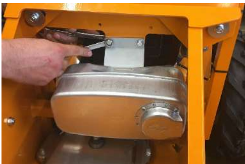
Demount the muffler
