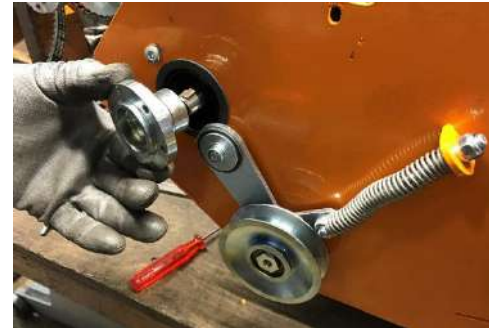
Pulled off belt pulley hub.
