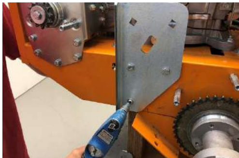
Tighten the central locking screw (Torx) with 25 Nm.
