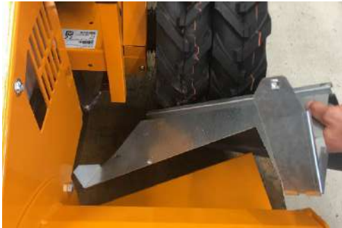
Demount the cover and rubber
