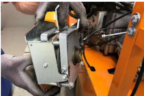
Taking off the steering-brake
