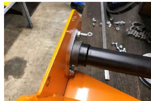
Unscrew and take out the angular gear unit.
