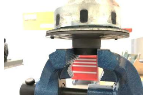
Clamp in clutch on the clutch hub. Not on the slide bearing!
