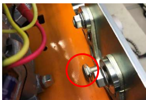
Insert long carriage bolt with washer.
