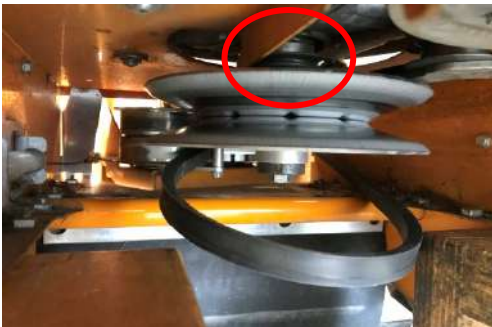
Take flail belt off of the rear belt pulley. Now the drive belt above can be taken off.
