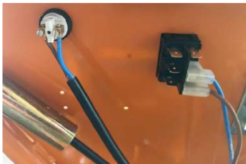
AS 901 cabling – handlebar with new start switch.
