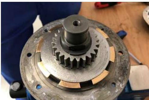
Then an inside disc (steel), etc.
