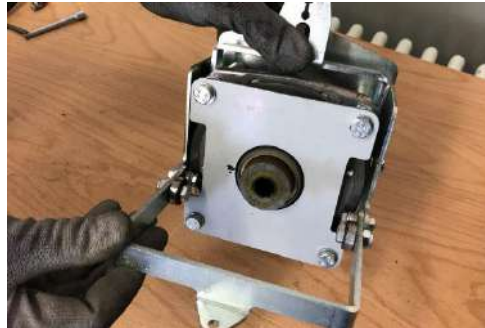
Steering-brake taken off.
