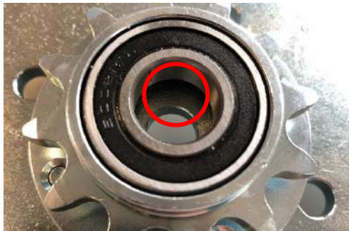
Do not forget the spacer
