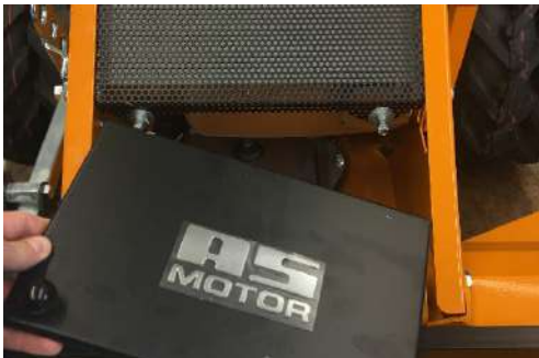
Remove the cover and heating shield
