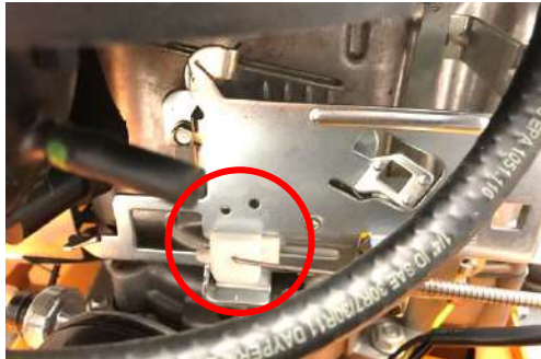
AS 701 SM: Idle position of the throttle lever.
