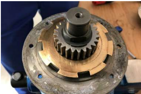
Reassembly of the clutch: First an outside disc (bronze)
