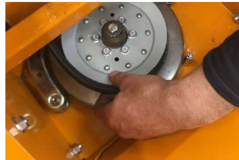
Remove the belt Demount the bowden cable of the blade clutch
