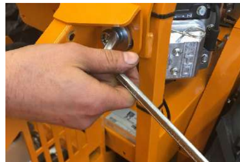
Remove the frame bolts on each side
