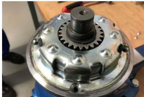
Insert apertures of the clutch basket precisely in the apertures of the disc pack.
