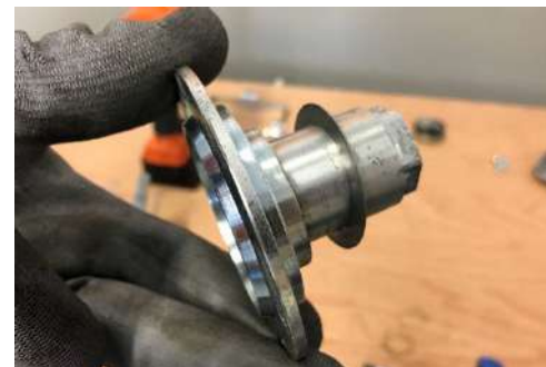
Pay attention to the O-ring when re-installing. (Not present for all machines)
