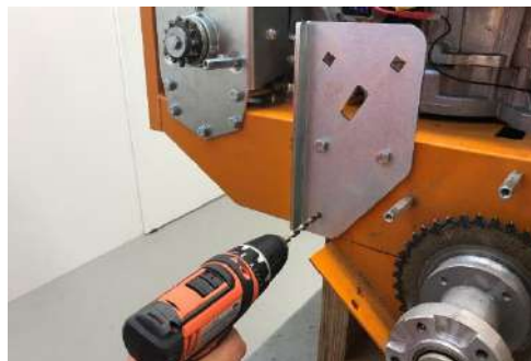
Drill a third hole with a 6 mm bit.
