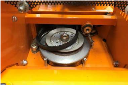
Take flail belt off of the belt pulley.
