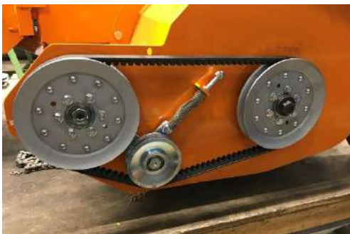
Belt drive of the flail shaft.
