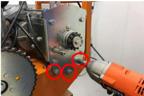
Unscrew three screws.
