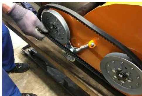
Take the belt off of the belt pulley of the angular gear.
