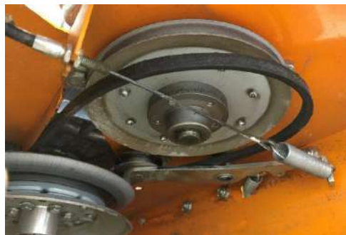
Take the drive belt off of the belt pulley.
