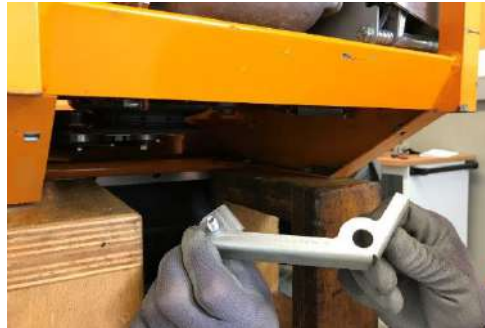
Unscrew the belt guide.
