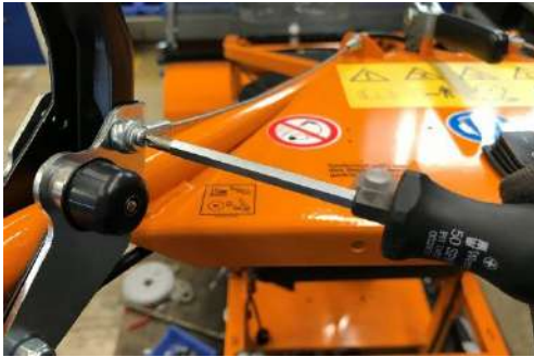
Fasten the cable on the lever
