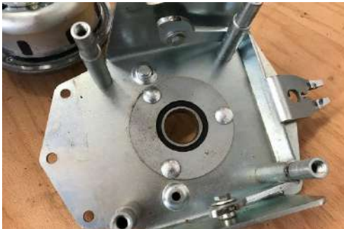
Clutch bearing. Check the ball bearing.
