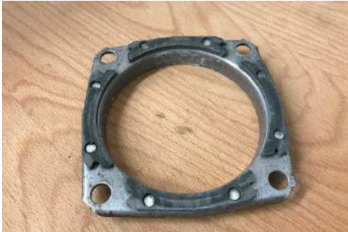
Brake plate with the four brake pads. Riveted.
