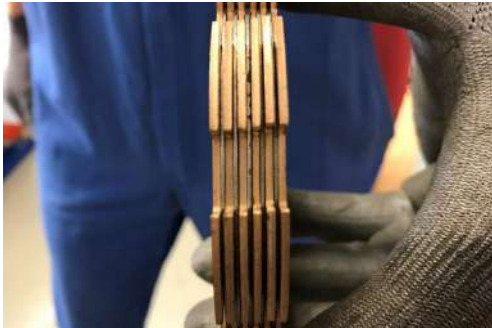
Stratification of the disc pack.
