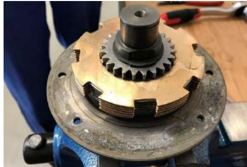
Stratified disc pack. Apertures of the discs one precisely above the other.
