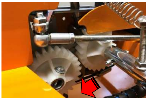
In MC mode, the gears are separated.
