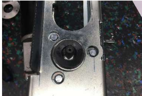
Mount the bearing and tighten the 3 bolts
