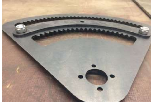
Steering quadrant reinforced s/n from February 2019
