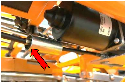
Tension spring pack tensions approx. 1 cm at activation of the lever to RC mode. (Ensures constant spring force and tension force)
