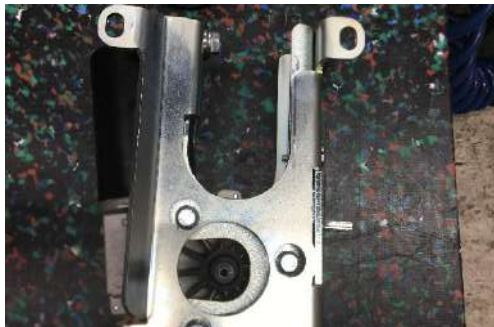
Remove bolts of the engine hub Remove engine hub and steering pinion
