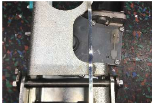
Remove locking switch
