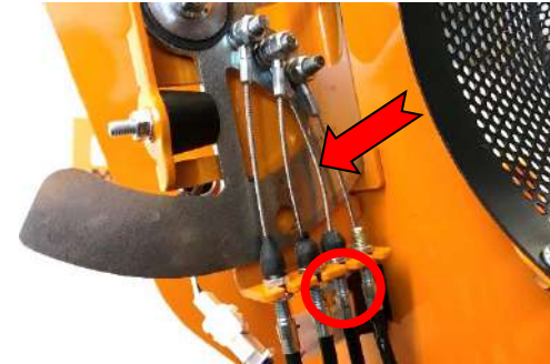
This cable moves the drive activation element in.
