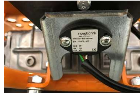
Angle sensor of the steering. Important: Notch of the position encoder in the direction of the cable. Rating plate visible.
