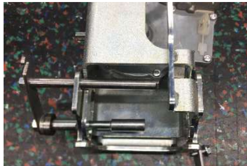
Remove bolts of the engine hub Remove engine hub and steering pinion
