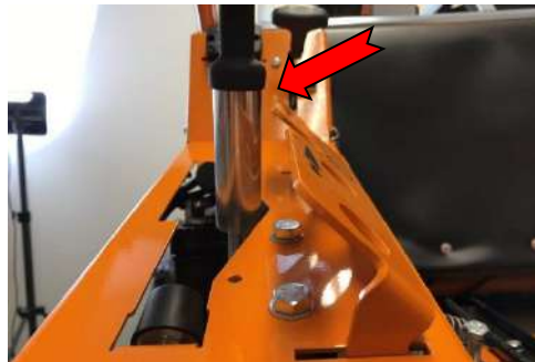
Tension spring pack tensions approx. 1 cm at activation of the lever to RC mode. (Ensures constant spring force and tension force)
