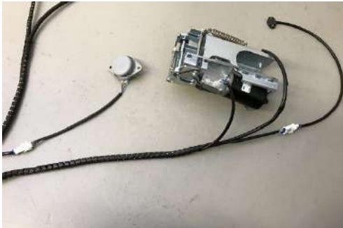
Steering activation element, angle sensor of the steering activation element and seat contact switch.
