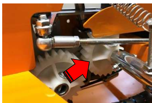
Cable 2: Drive lever clutch Engages gears of the drive lever actuator in RC mode. Can be adjusted on both cable stops.
