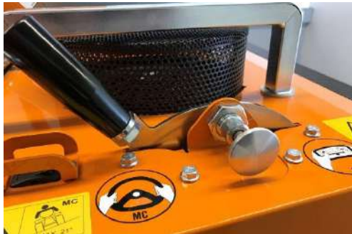
The changeover lever of the operating modes MC/RC. (manual control/remote control)
