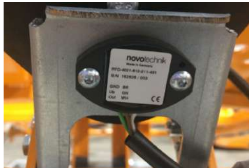
Steering Sensor bracket reinforced s/n from February 2019
