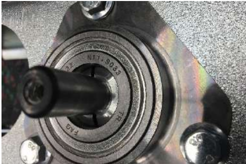
Mount the bearing and tighten the 3 bolts
