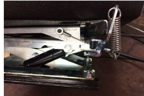
The new spring package has a Bowden cable that moves the drive lever into middle position when no one is sitting in the seat.
