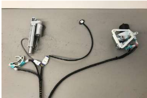
Cutting height actuator with cutting height detection and blade clutch activation.
