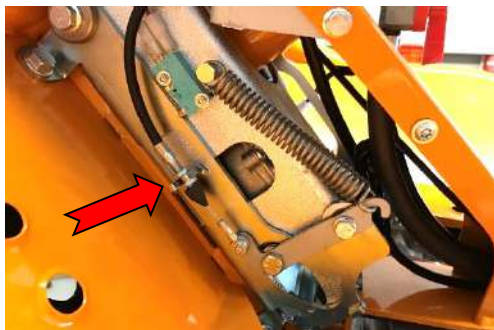
Cable 1: Steering clutch Activates mechanism of the steering clutch. Can be adjusted on both cable stops.
