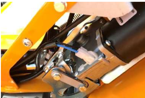
Power supply of the gear motor.
