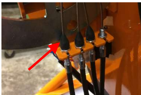
Detach Bowden cable on the MC - RC changeover and remove cable
