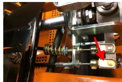
Install Bowden cable on the drive lever activation element
