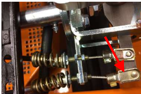
Detach the Bowden cable on the drive lever activation element
