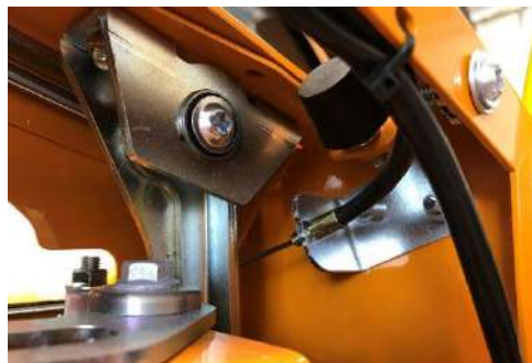
Adjustment only on one cable stop possible. Only on the changeover lever. Other cable stop is fixed. (Illustration)
