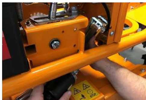
Take out drive lever activation in this position.
