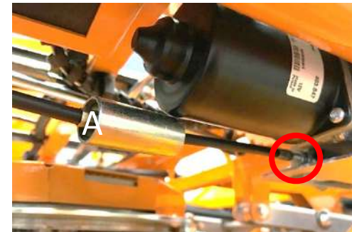
At RC mode the drive activation element moves the gear in.
