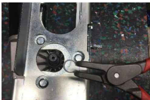
Remove locking ring
