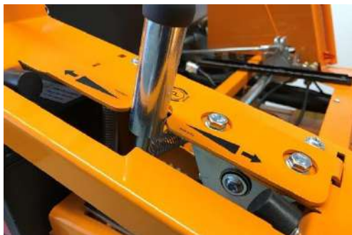
Cable 3: Drive lever gate When switching to RC mode the shift gate of the drive lever lifts.
