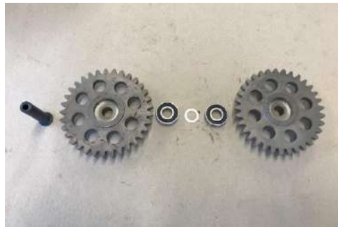
Fit together both double gears 12/33 teeth with two bearings, feather key and gear axle.
