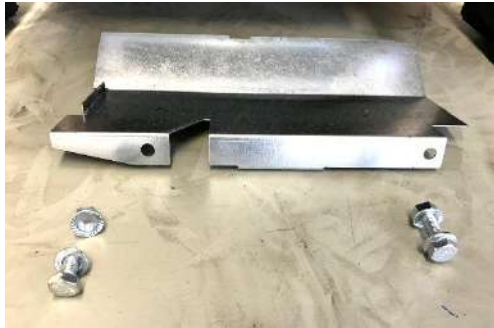
Removed hand guard with both screws.
