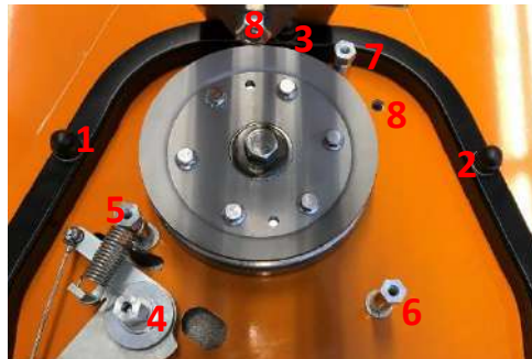
View of the blade enclosure from above. Position of the screws of the blade bearing.
