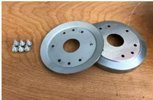
Removed belt pulley with lower brake drum.
