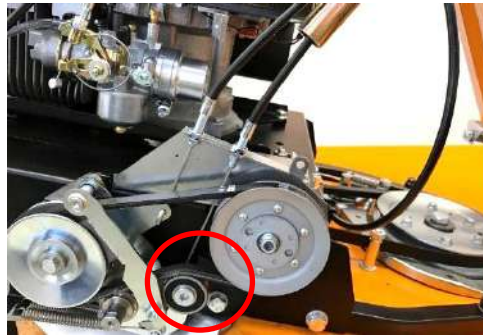
Tensioned drive belt at activated drive lever.
