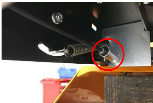
Bowden cable of the blade clutch with integrated compression spring package.
