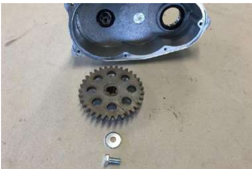
Fasten 33-tooth on the gear shaft with screw and washer.
