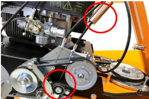
Integrated spring package of the cable. The traction drive cable tensioned via the tensioning lever of the drive belt.
