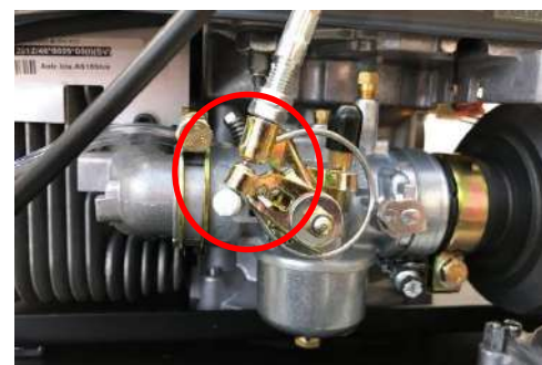
Position of the accelerator cable at "full throttle".
