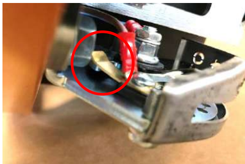
In the throttle lever position "Off" the throttle lever touches the short-circuit contact.
