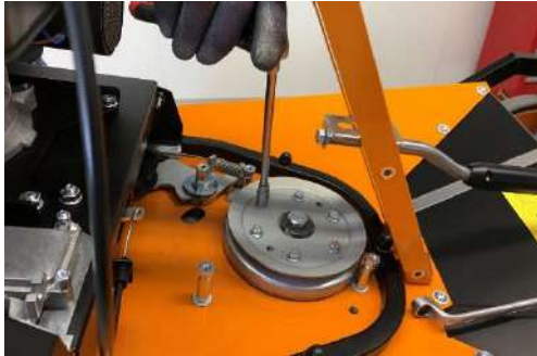
Unscrew the belt pulley.
