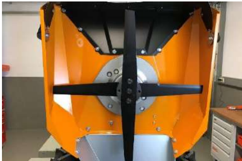
Cross-blade system of the AS 63.
