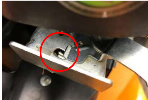
Position of the accelerator cable at "idle". Throttle lever no longer touches the short-circuit contact.
