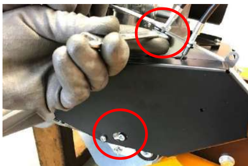
The parking brake is adjusted on the cable stop.
