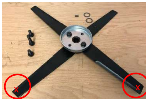
Resharpener and balance blades uniformly. Imbalance can damage the machine and the engine. Do wear or resharpen the blades beyond the wear marks (grain markings "dot" on positions "x").
