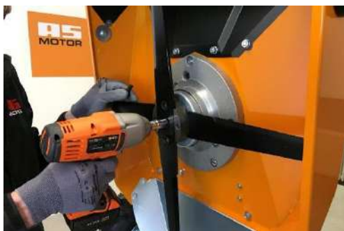
Take off blade. Tightening torque at installation: 120 Nm. ⚠
