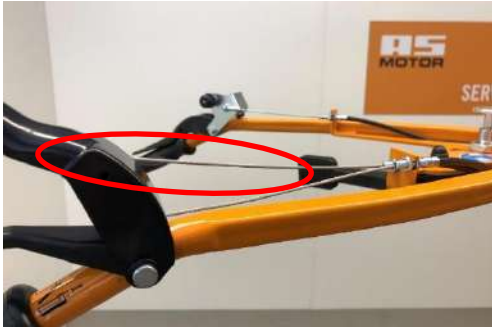
The drive lever, right with, traction drive cable.
