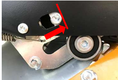
When activating the brake lever, the parking brake opens.
