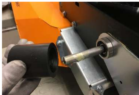
Remove the grass winding protection
