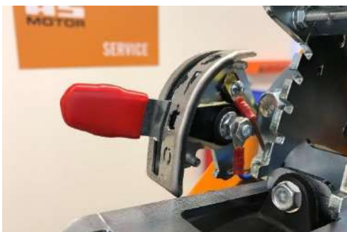
Throttle lever position: "Idle position"
