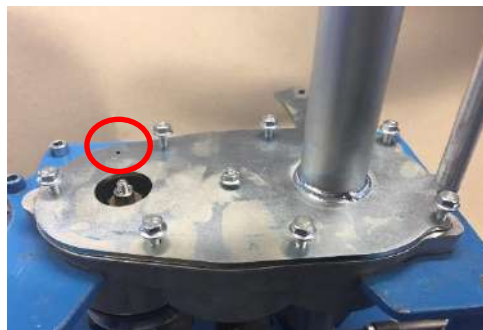
Drive gear assembly with belt pulley. Do not forget the feather key.
