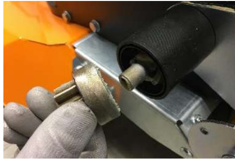
Pull off the left drive pinion
