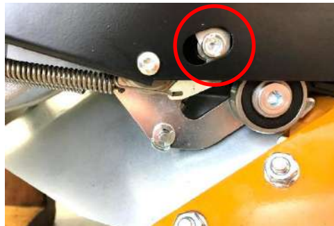
With the parking brake closed, there is a gap between screw head and belt guard.
