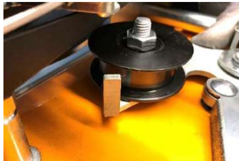
Tensioning roller of the blade clutch with belt tensioner.
