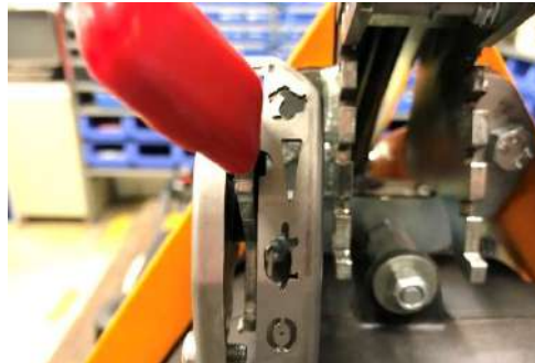
Throttle lever position: "Full-throttle". The B&S 850 E I/S does not have a choke position on the throttle lever.
