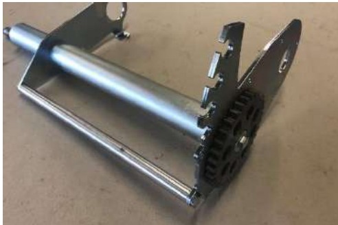
Fastened strut and 33-tooth gear.
