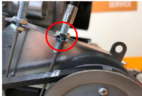
Integrated spring package of the cable. The traction drive cable tensioned via the tensioning lever of the drive belt.
