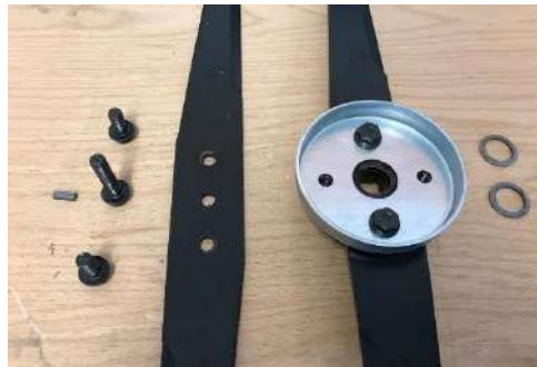
The blade system and its component parts.
