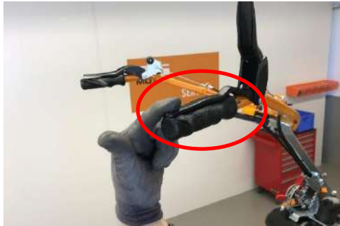
When activating the brake lever, the parking brake opens.
