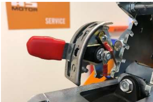
Throttle lever position: "Idle position"
