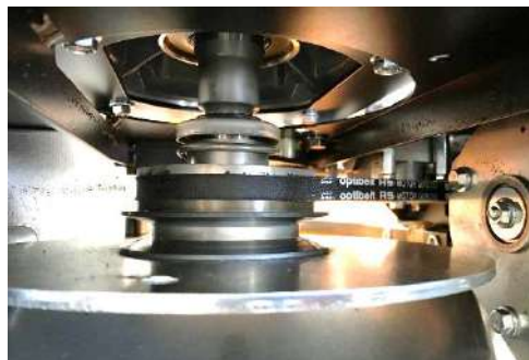
The, take off the Variomat drive belt. It goes from the Variomat to the angular gear unit.
