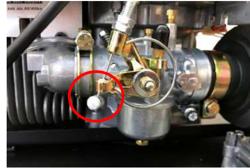
Position of the accelerator cable at "idle".
