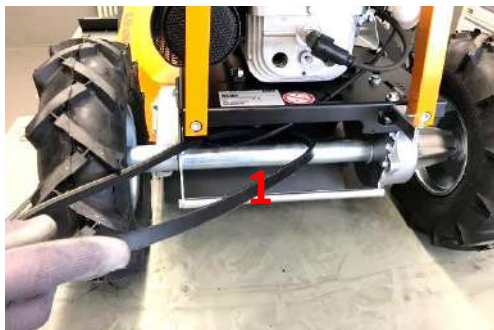
Pull out blade belt over the axle and to the rear.
