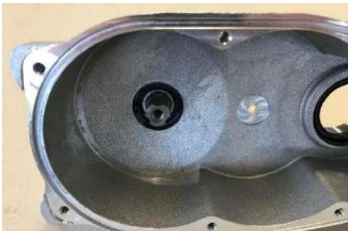
Installed wheel shaft.
