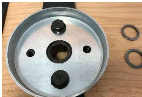
Wrap protection cup with lock screws of the upper mulching blade.
