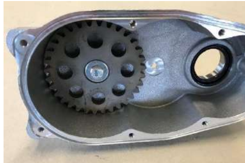
Mounted gear. The gear must not grind on the housing. If it does there is a material fault on the housing.
