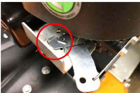
Position of the accelerator cable at "off". Throttle lever touches the short-circuit contact.
