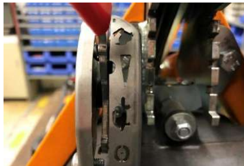
Throttle lever position: "Start/Choke". The Honda GXV 160 always needs the maximum choke when starting. If the choke is not closed 100%, start problems occur.
