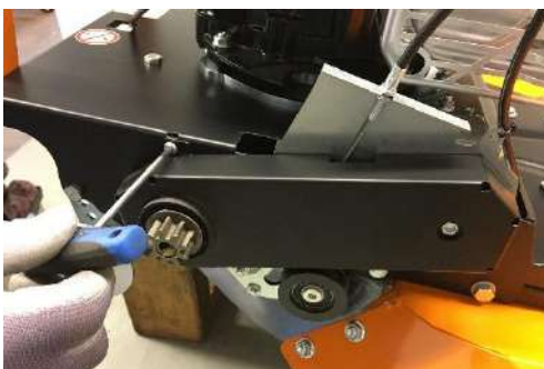
Loosen the screws of the belt cover Remove the belt cover
