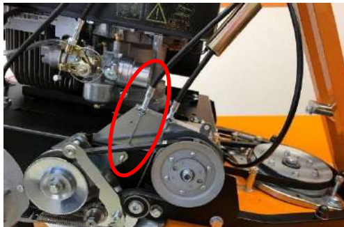
The Bowden cable is fastened on the brake lever.
