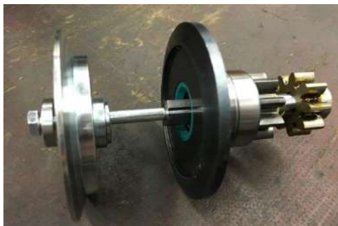
Drive gear assembly with belt pulley. Do not forget the feather key.
