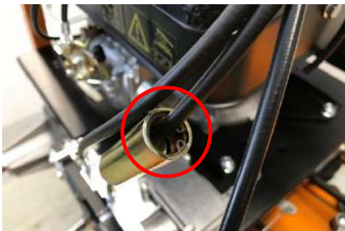
When activating the drive lever, the spring package of the cable must deflect by approx. 1.5 – 2.0 cm.
