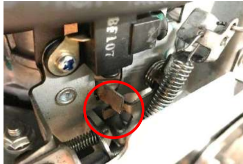
Position of the accelerator cable at "full throttle". Throttle lever lightly touches the choke lever, without lifting it.
