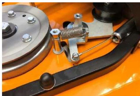
The tensioning lever of the blade clutch must be taken off.
