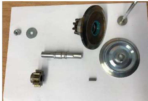
Component parts – drive gear with belt pulley.
