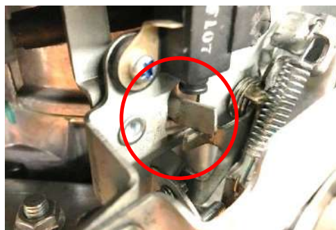
Position of the accelerator cable at "Start/Choke". Throttle lever touches the choke lever and pushes it all the way up. Choke is closed 100%.
