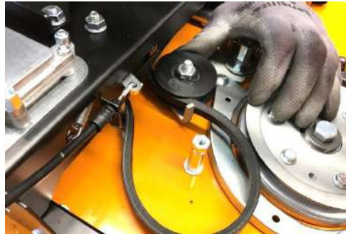
To do this thread the blade belt out of the belt guide of the tension roller. With your hand, pull the tensioning roller under the engine mount.
