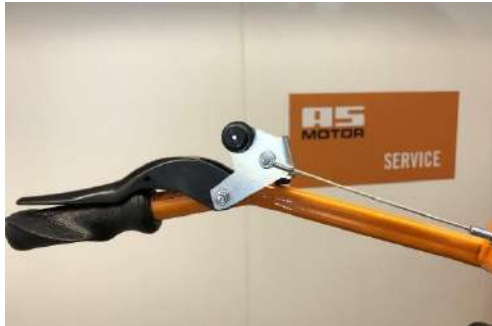
Lever of the blade clutch with Bowden cable on the left-hand side.
