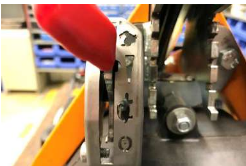
Throttle lever position: "Full-throttle"
