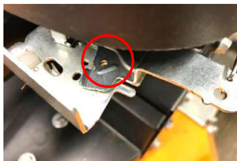
Position of the accelerator cable at "full throttle". Perforation of the throttle lever corresponds to the perforation of the sheet metal.
