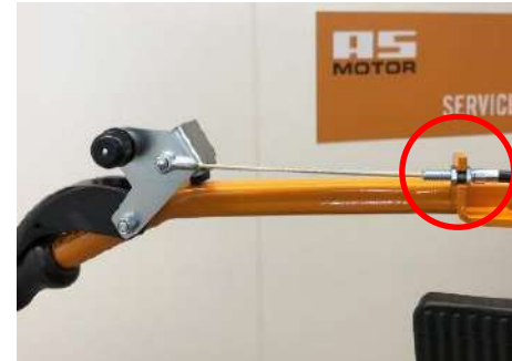
Lever of the blade clutch with Bowden cable on the left-hand side.
