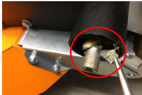
Pull the drive shaft to the left side Remove the carrier from the drive shaft
