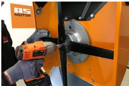
Unscrew central locking screws.
