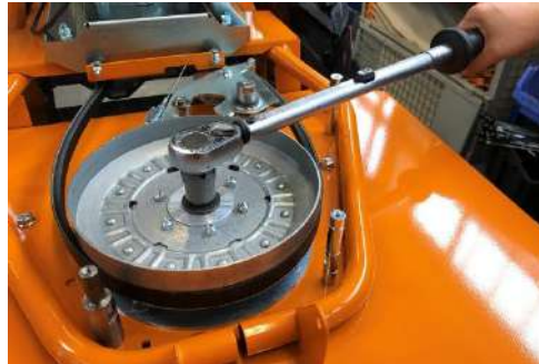
Unscrew the fastening screw of the belt pulley. To do this block the blade. (Note: Tightening torque 120 Nm! )
