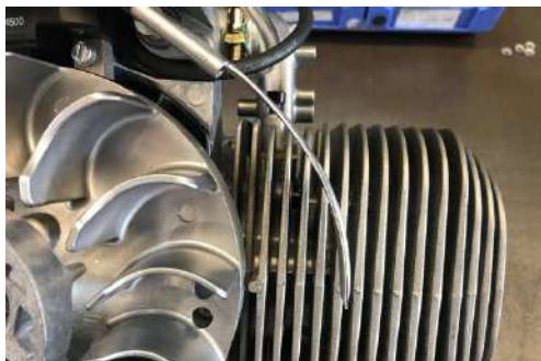
Position of the wind vane (mechanical regulator) at minimum petrol (throttle flap almost closed).
