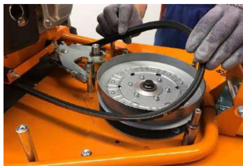
Pull the belt off of the belt pulley.
