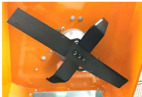
Take off blade. (Note: Tightening torque of the locking screws of the blade 120+5 Nm! ) ⚠
