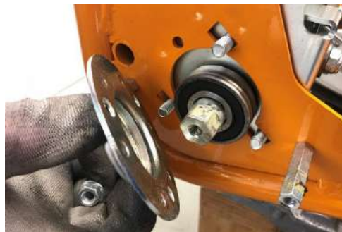
Unscrew bearing plate and take out the ball bearings. Check the ball bearing.
