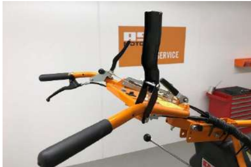
The drive lever is on the right side of the handlebar.
