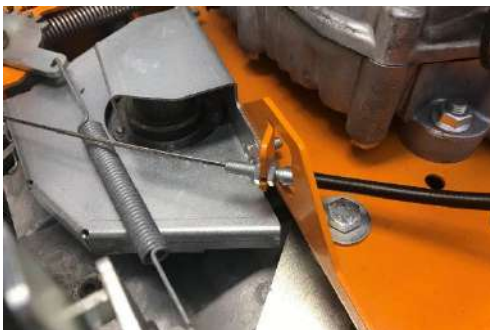
Factory setting of the lower cable stop.
