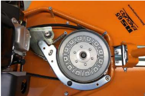
View of the blade clutch, blade brake, belt pulley and blade belt.
