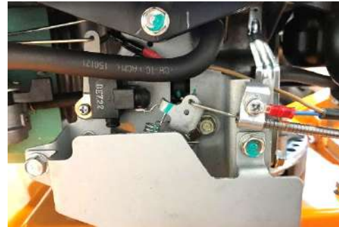
Cabling: Blue cable on the cable stop. Brown cable on the black cable and then to the ON/OFF switch.
