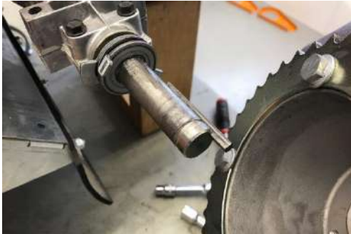
Pull off wheel hub. Take off the long feather key and thrust washers.
