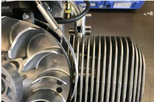
Position of the wind vane (mechanical regulator) at full throttle (throttle flap completely opened).
