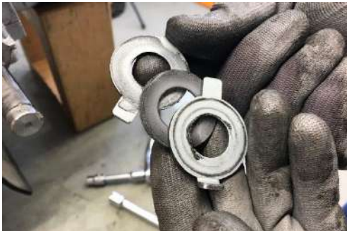
Sequence of the three thrust washers.
