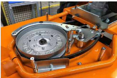
Unhook tension spring of the engine brake and take off the brake lever.
