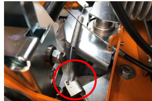
.....Tensioning pulley lever of the drive not tensioned.
