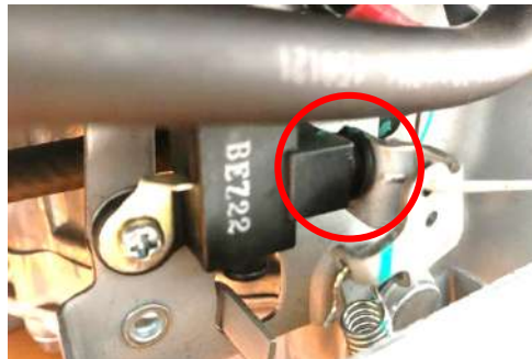
AS 65 4T Honda: Bring throttle lever into zero position. Limit switch pressed. The limit switch has no function, because there is the ON/OFF switch on the handlebar.
