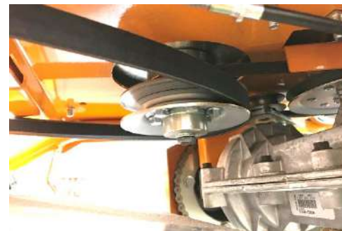
Blade belt is now free and can be replaced.
