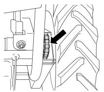
The chains on the right and left of the differential lock must be lubricated on a regular basis. We recommend the use of biodegradable chain spray.
