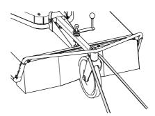
Secure the device with belts to the frame elements that can hold the weight.
